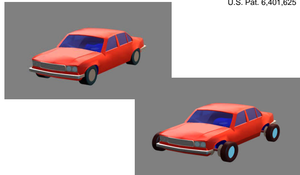
MegaRail dualmode car wheels shift out to allow wheels to operate inside rails
