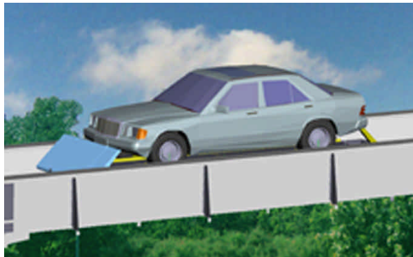
MegaRail car ferries carry standard cars with driver and passengers inside
