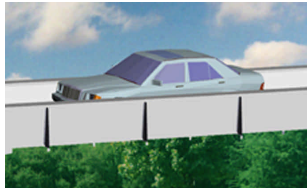
MegaRail dualmode electric cars use both automated guideway & city streets
